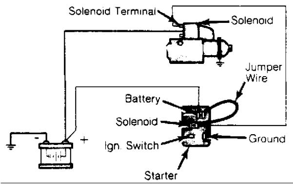
Fig. 1: Typical Starter Solenoid Test
